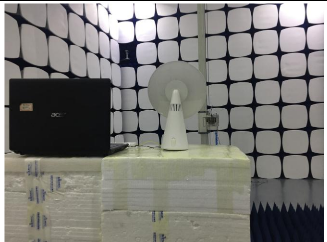
Radiated Spurious Emissions Test Setup Above 1GHz
