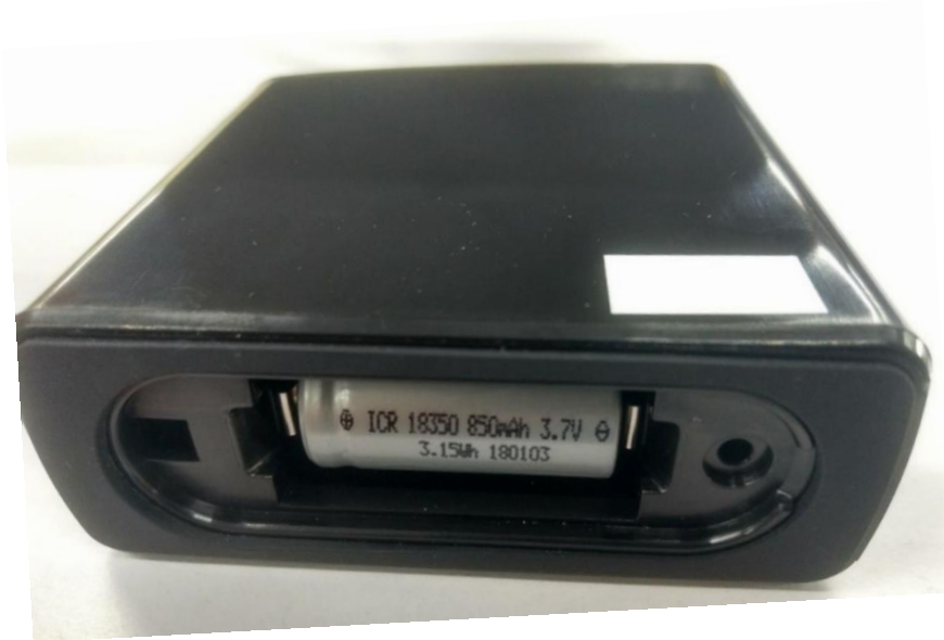
Figure 6 – Li-ion battery compartment and placement with polarity
