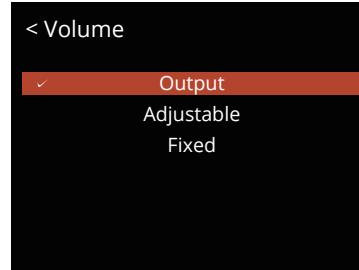
When set to ADJUSTABLE, the D9 Volume control is used to adjust the level of the analogue output. This is required when connecting directly to a power amplifier. The default setting on the D9 is ADJUSTABLE.
