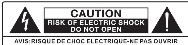
This lightning flash with an arrowhead symbol within an equilateral triangle is intended to alert the user to the presence of non-insulated "dangerous voltage" within the product's enclosure that may be of sufficient magnitude to constitute a risk of electric shock.
