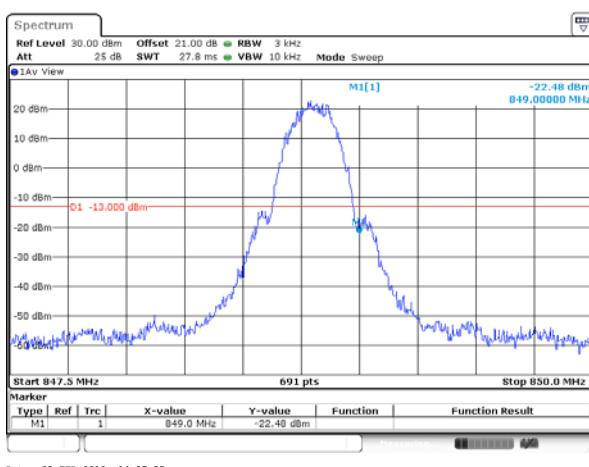
Conducted Band Edge plot on channel 810
