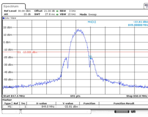
Conducted Band Edge plot on channel 810
