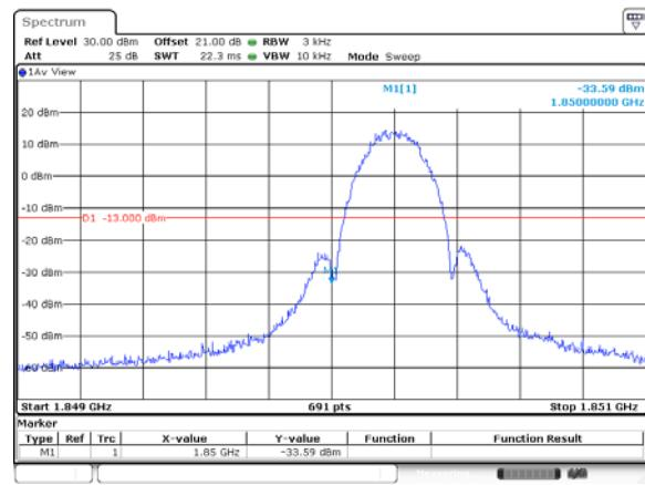
Conducted Band Edge plot on channel 251
