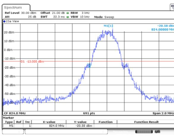
Conducted Band Edge plot on channel 810
