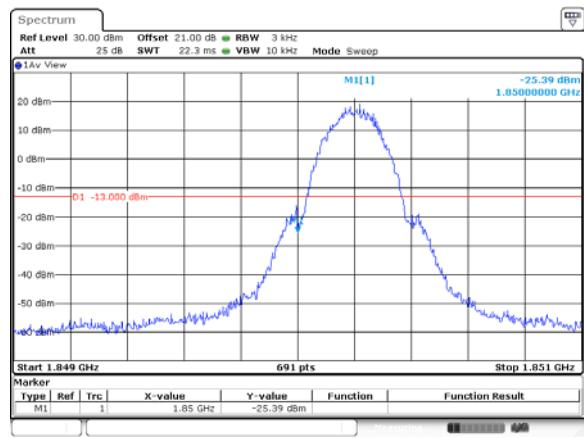
Conducted Band Edge plot on channel 251
