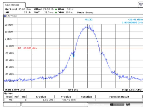
Conducted Band Edge plot on channel 251
