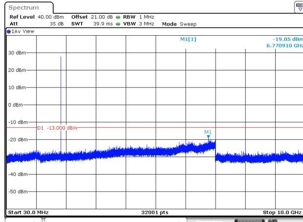
Conducted Emission Transmitting Mode CH 251
