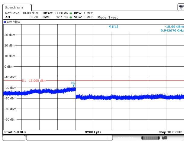
Conducted Emission Transmitting Mode CH 190
