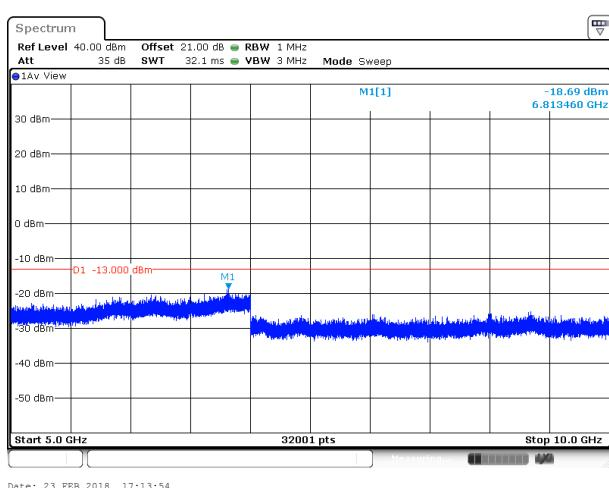
Conducted Emission Transmitting Mode CH 190
