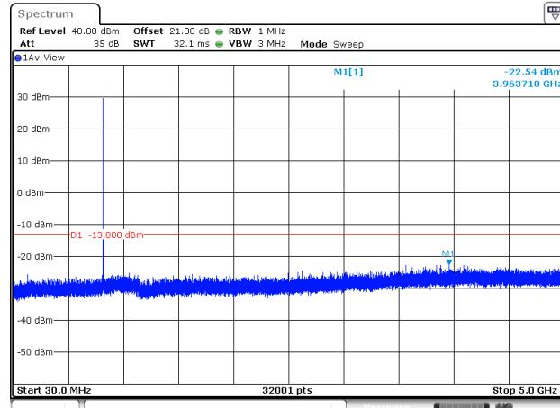
Conducted Emission Transmitting Mode CH 128
