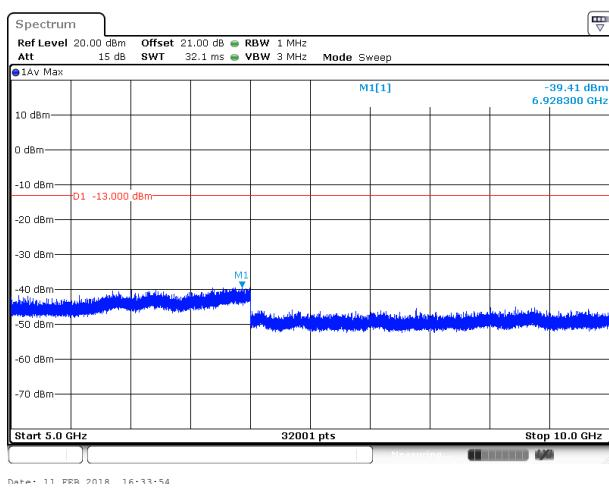
Conducted Emission Transmitting Mode CH 4183
