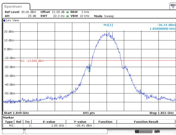
Conducted Band Edge plot on channel 251
