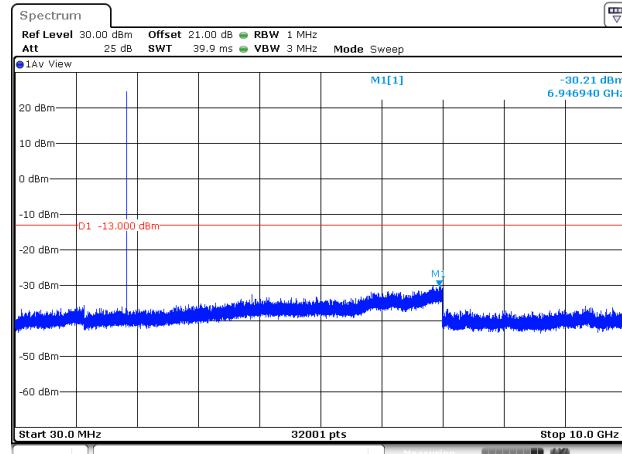
Conducted Emission Transmitting Mode CH 251
