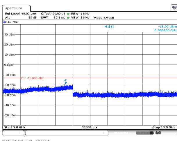
Conducted Emission Transmitting Mode CH 512
