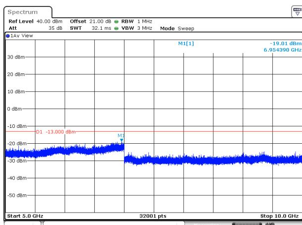
Conducted Emission Transmitting Mode CH 512
