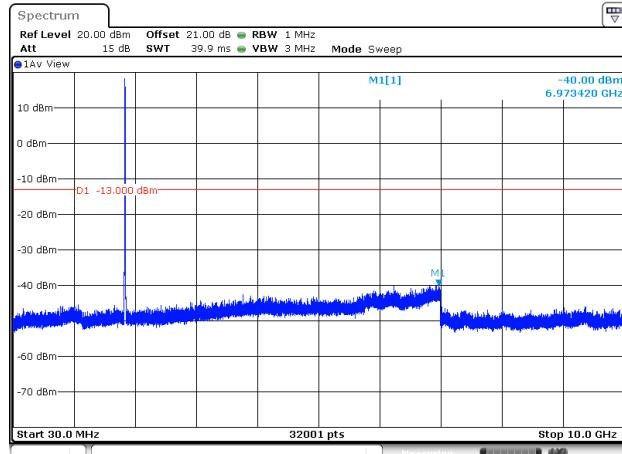
Conducted Emission Transmitting Mode CH 4233
