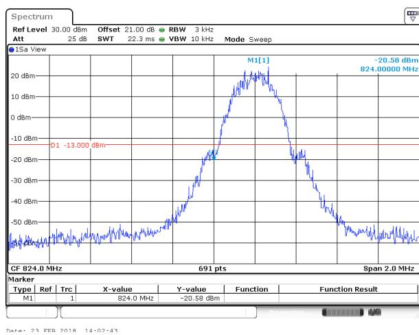
Conducted Band Edge plot on channel 810
