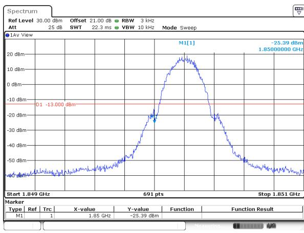
Conducted Band Edge plot on channel 251
