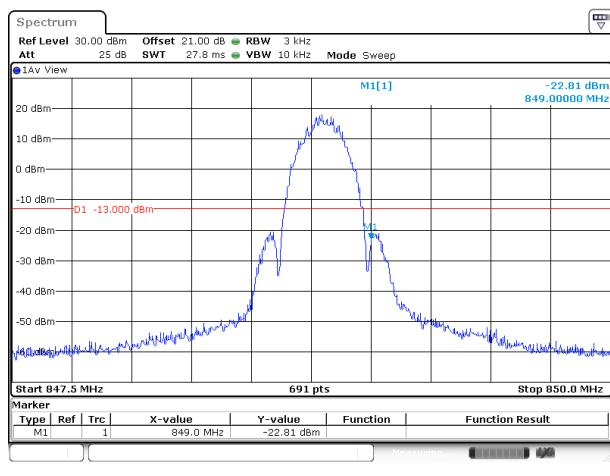
Conducted Band Edge plot on channel 810
