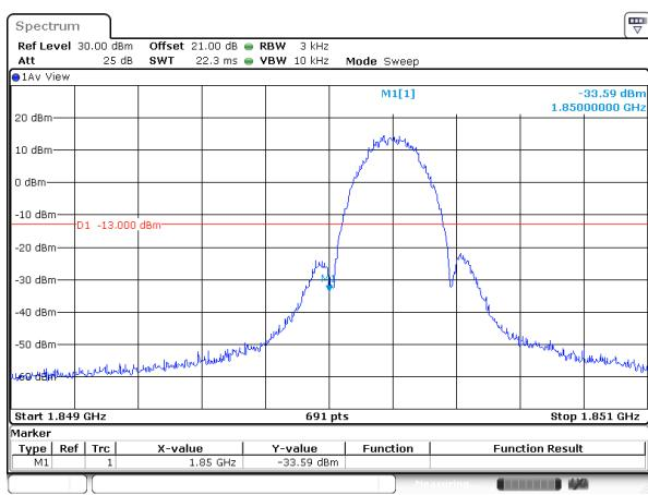
Conducted Band Edge plot on channel 251
