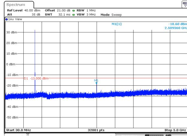
Conducted Emission Transmitting Mode CH 128
