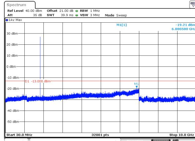
Conducted Emission Transmitting Mode CH 251
