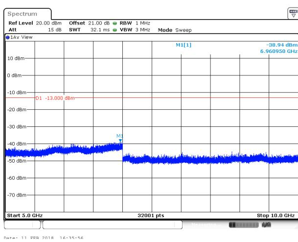
Conducted Emission Transmitting Mode CH 9262
