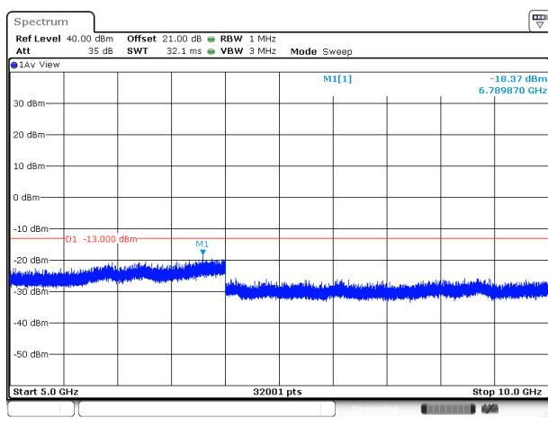
Conducted Emission Transmitting Mode CH 190
