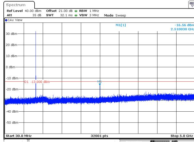
Conducted Emission Transmitting Mode CH 128
