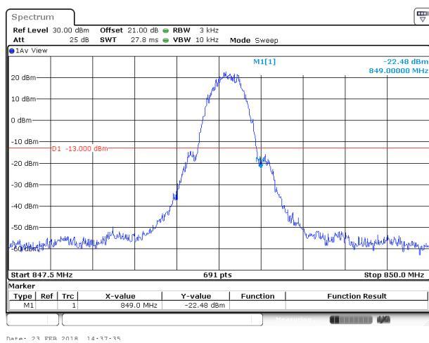
Conducted Band Edge plot on channel 810
