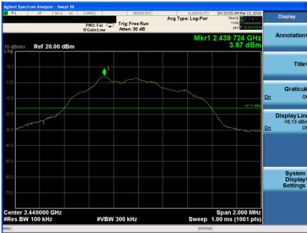
GFSK on channel 19
