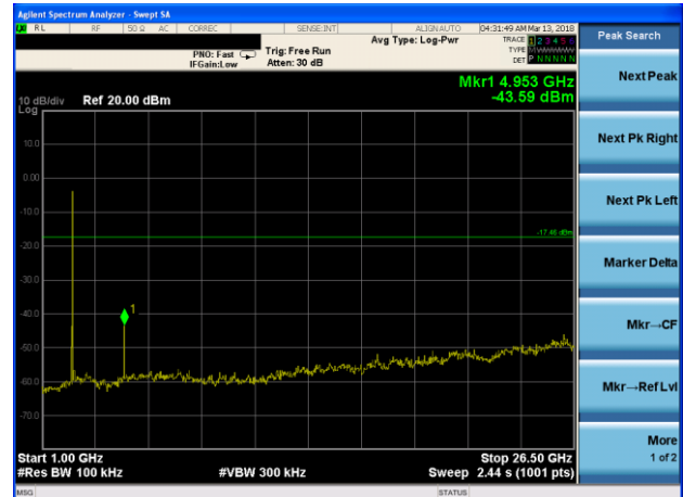
GFSK on channel 39
