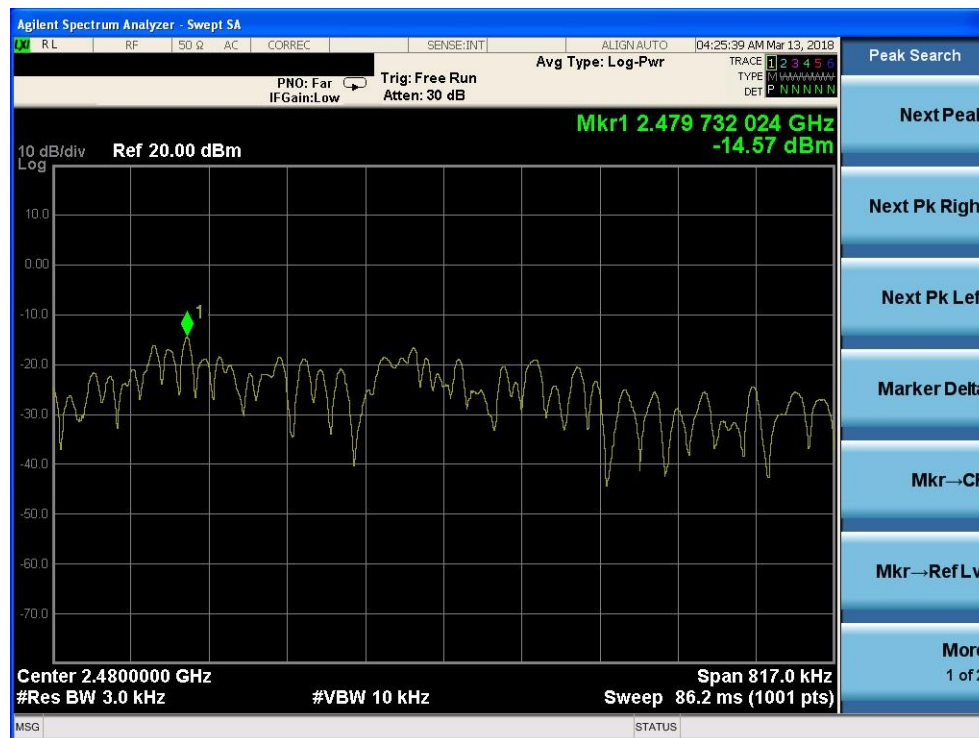
Power spectral density plot on channel 39
