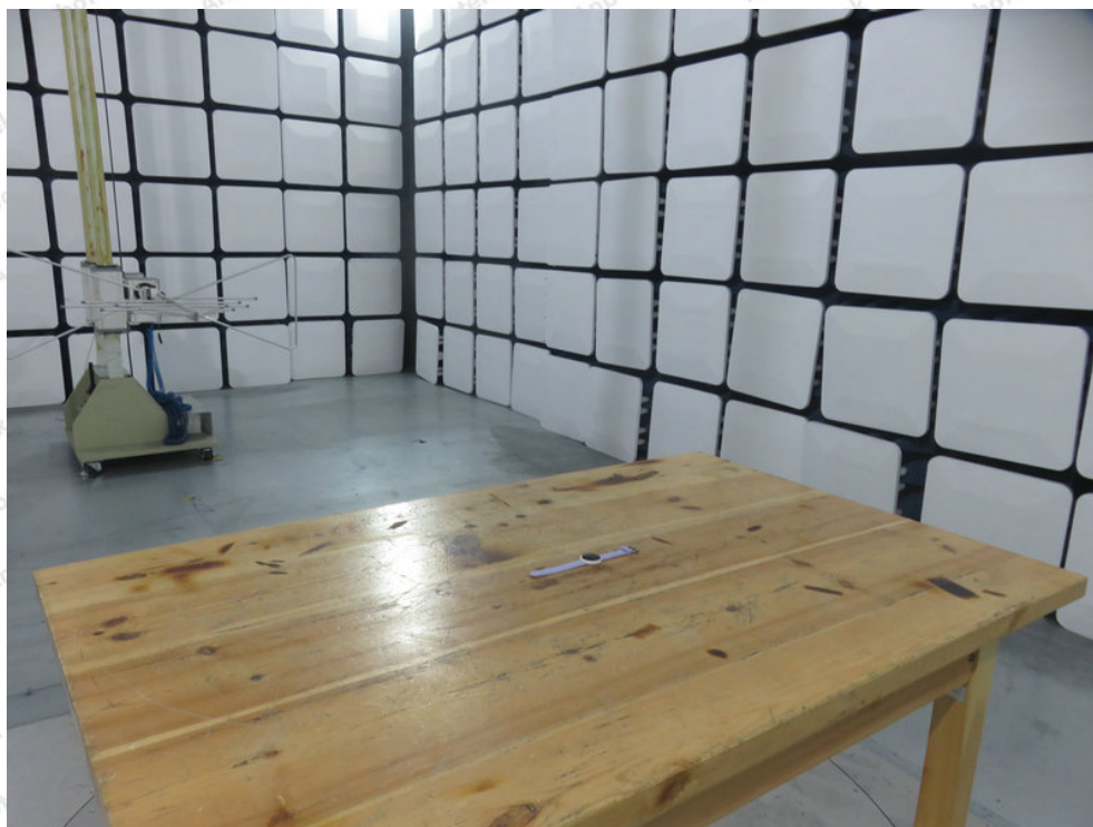
Photo of Radiation Emission Test
