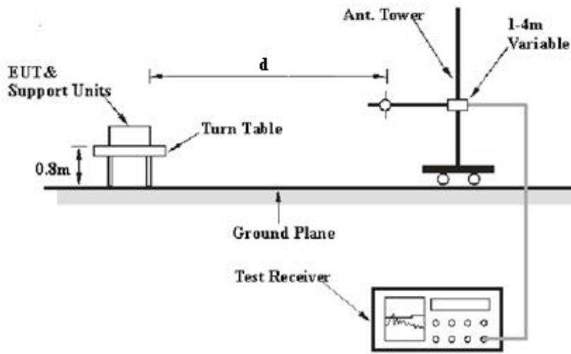
The radiated emission tests were performed at the 3 meters distance, using the setup accordance with the ANSI C63.4-2014. The specification used was the FCC Part 15.109 Class B limits.
