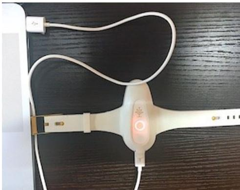
With the microUSB cable included in the package, connect the controller with your computer.
