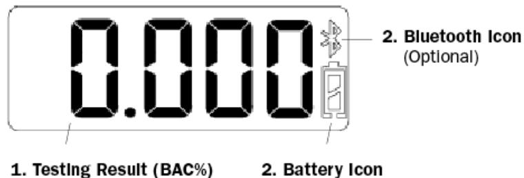
**NOTE:** The battery icon will flash when the battery is low indicating it is time to recharge. If the battery capacity is too low the tester will not turn on. The Bluetooth indicator will illuminate when the optional *Smart Phone Data Collection* application is active.
