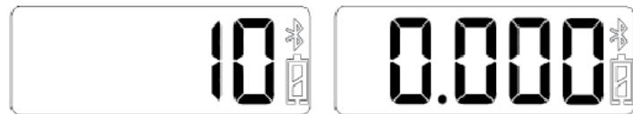
5. If the *LCD Display* shows "Err0" this is an error message and an indication that there was an insufficient breath flow rate or an interruption in the blowing. Please resubmit your breath sample. If the breath sample is successful the *Display* will show the Breath Alcohol Concentration as a percentage value.
