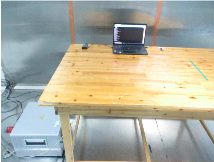
Photograph 2: Set-up for measurement of radiated emission
