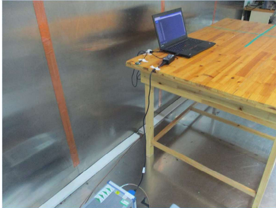
Photograph 1: Set-up for measurement of conducted emission
