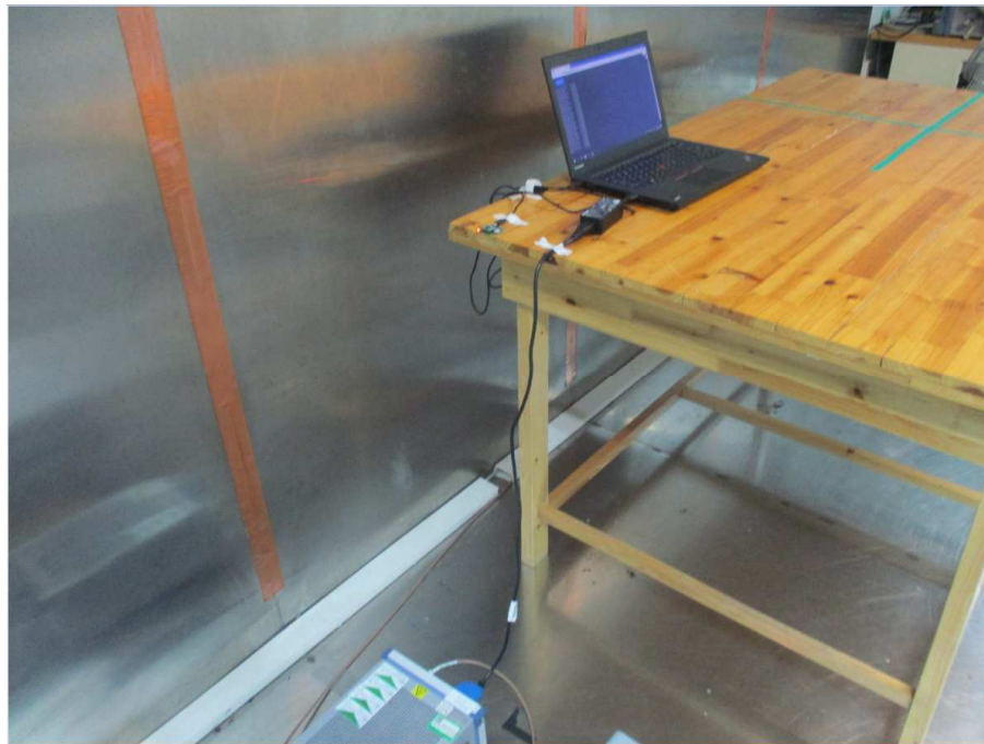
Photograph 1: Set-up for measurement of conducted emission
