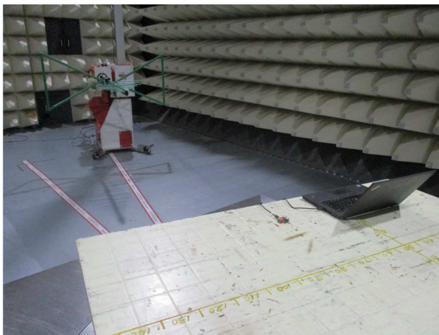
Photograph 2: Set-up for measurement of radiated emission
