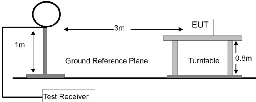
For Radiated Emission 30-1000MHz
