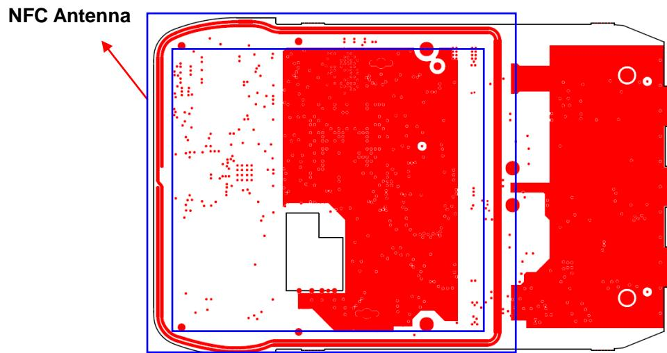
**Note: PCB board is multi-layer board and NFC antenna is integrated on PCB**
