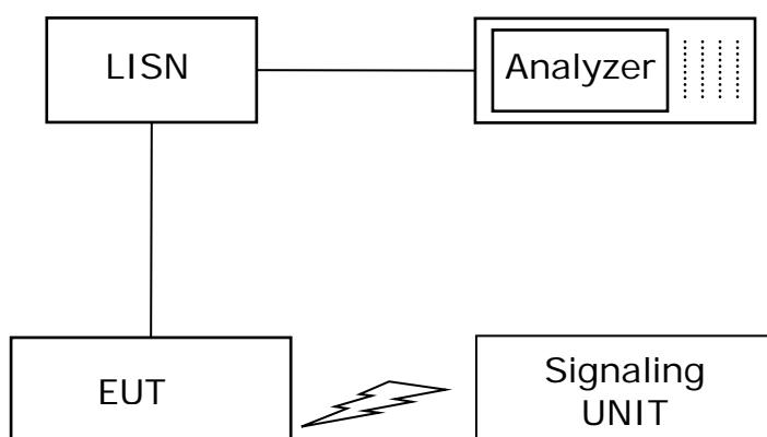
Setup in the shielded room for conducted measurements at AC mains port
