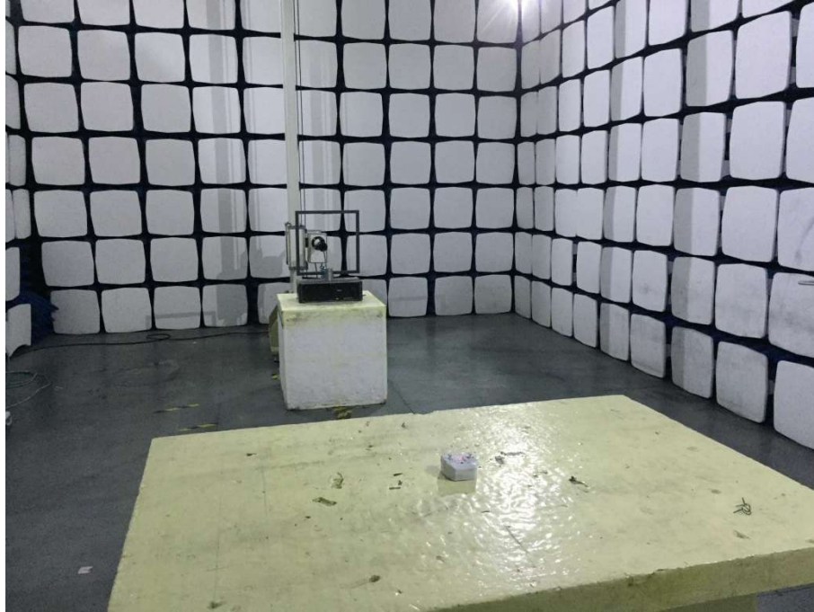
Radiated Emission Test Setup (Below 30 MHz) from 0.8M-Height Turntable Test Table
