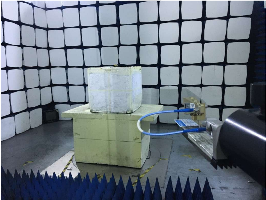
Radiated Emission Test Setup (Above 18 GHz) from 1.5M-Height Turntable Test Table
