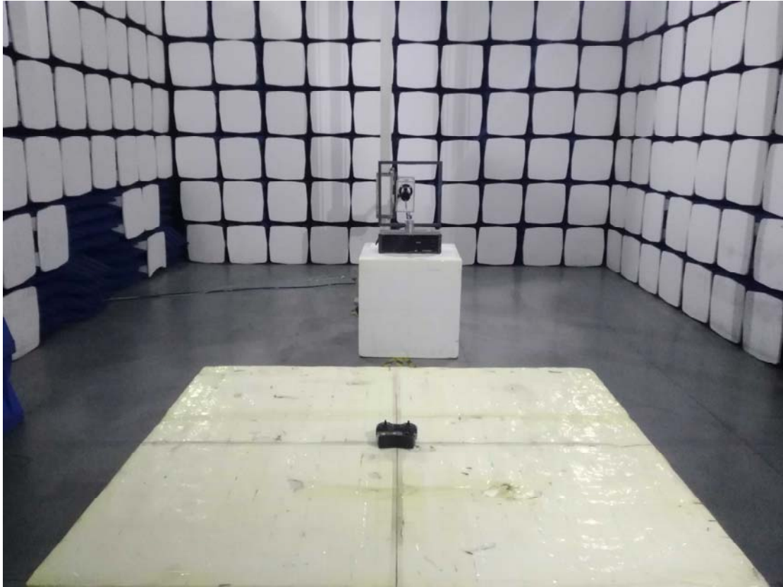
Radiated Emission Test Setup (from 9 kHz to 30 MHz) from 0.8M-Height Turntable Test Table
