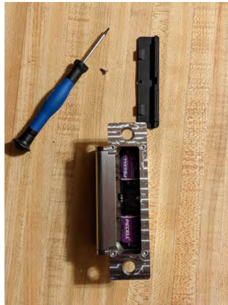
Remove Black Cover Remove Batteries by hand, Install new batteries with (+) terminal pointing towards each other
