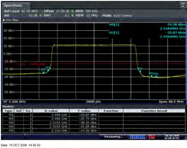
Figure 8.2-57: Conducted band edge emissions for 64QAM 2506 MHz, 20 MHz channel - Port 1
