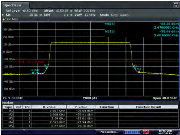
Figure 8.2-63: Conducted band edge emissions for 64QAM 2680 MHz, 20 MHz channel - Port 1
