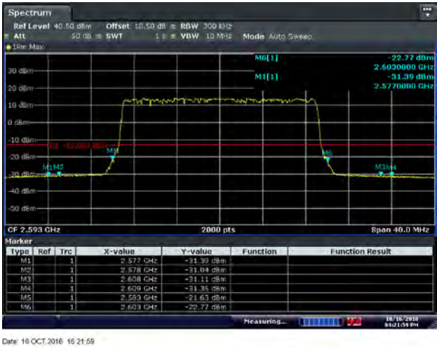
Figure 8.2-59: Conducted band edge emissions for 16QAM 2593 MHz, 20 MHz channel - Port 1
