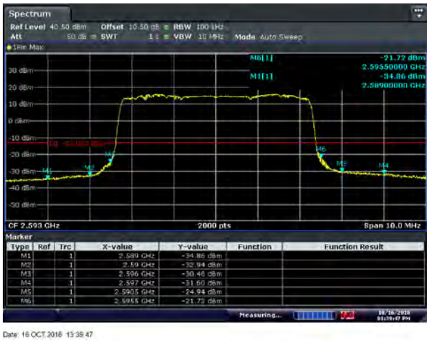
Figure 8.2-41: Conducted band edge emissions for 16QAM 2593 MHz, 5 MHz channel - Port 1
