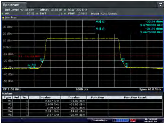
Figure 8.2-61: Conducted band edge emissions for QPSK 2680 MHz, 20 MHz channel - Port 1
