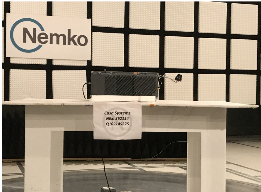
Figure 8.1-4: Radiated measurement setup photo
