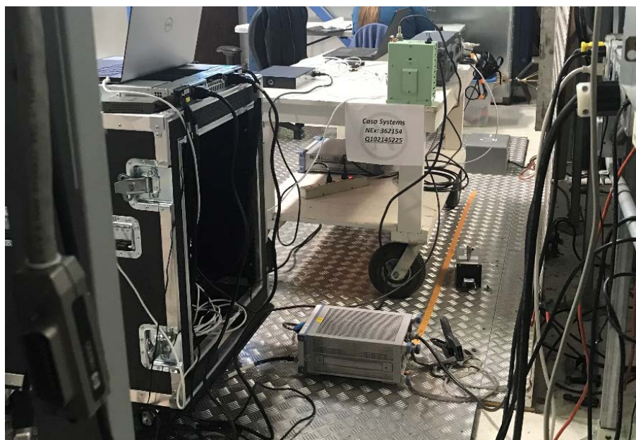
Figure 8.2-4: Conducted disturbance at mains port setup photo
