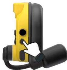
Push 'M' button to activate/deactivate mute.
