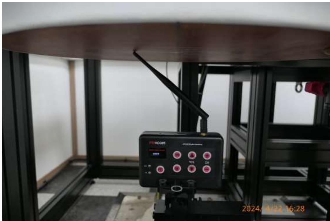
Top from ELI Phantom (Separation Distance: 0 cm) – Ant. 45 degrees
