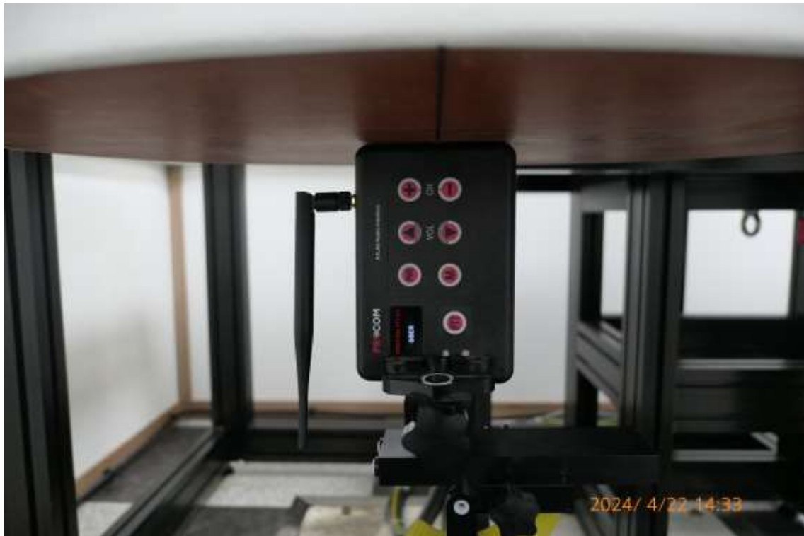
Right from ELI Phantom (Separation Distance: 0 cm) – Ant. 90 degrees
