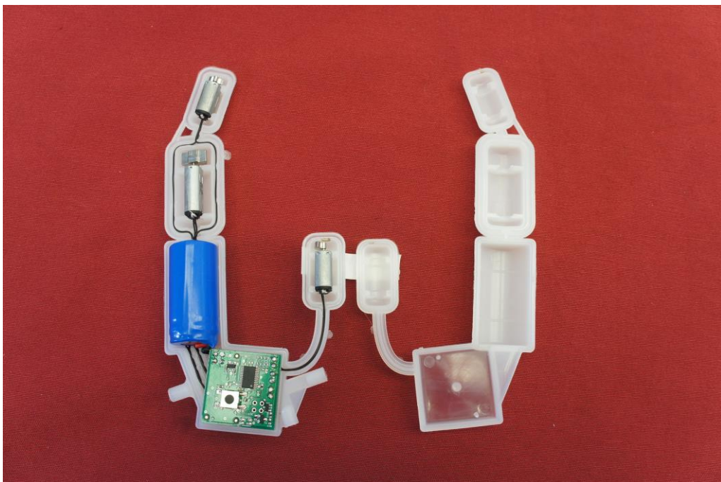
Picture 4: Opened host with RF module
