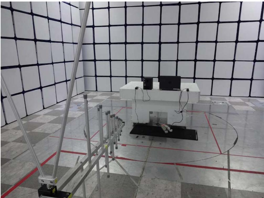
**Radiated disturbance at (1 ~ 6) GHz \_Test setup photo**
