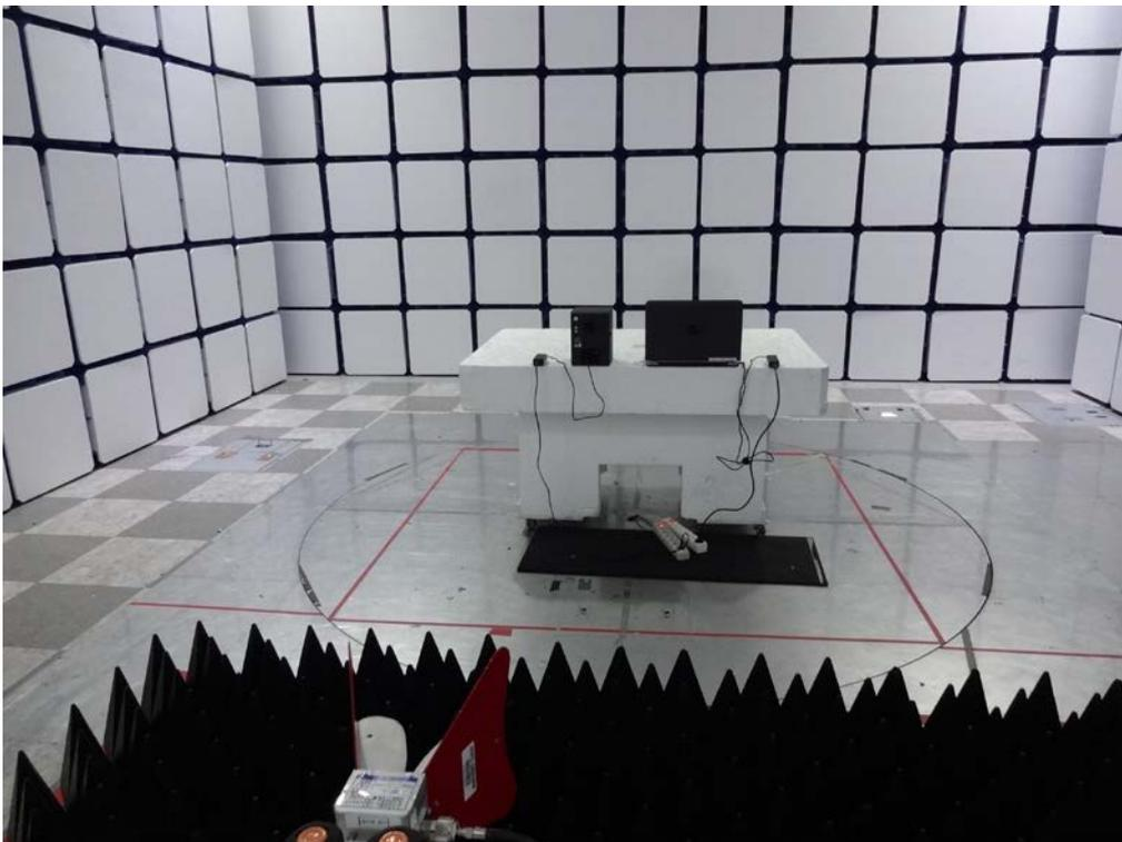
Radiated disturbance at (6 ~ 18) GHz \_Test setup photo
