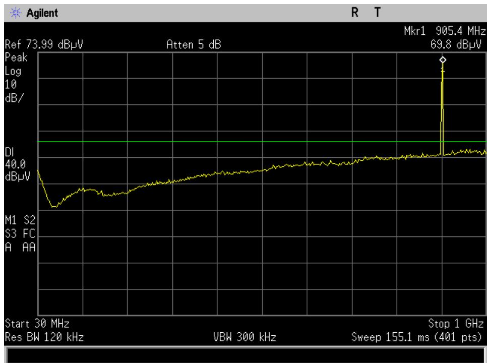
This plot is showing the emissions from the radio without any support equipment. The support equipment was needed to control the radio for testing and was the cause of the emissions from 30 MHz to 600 MHz.
