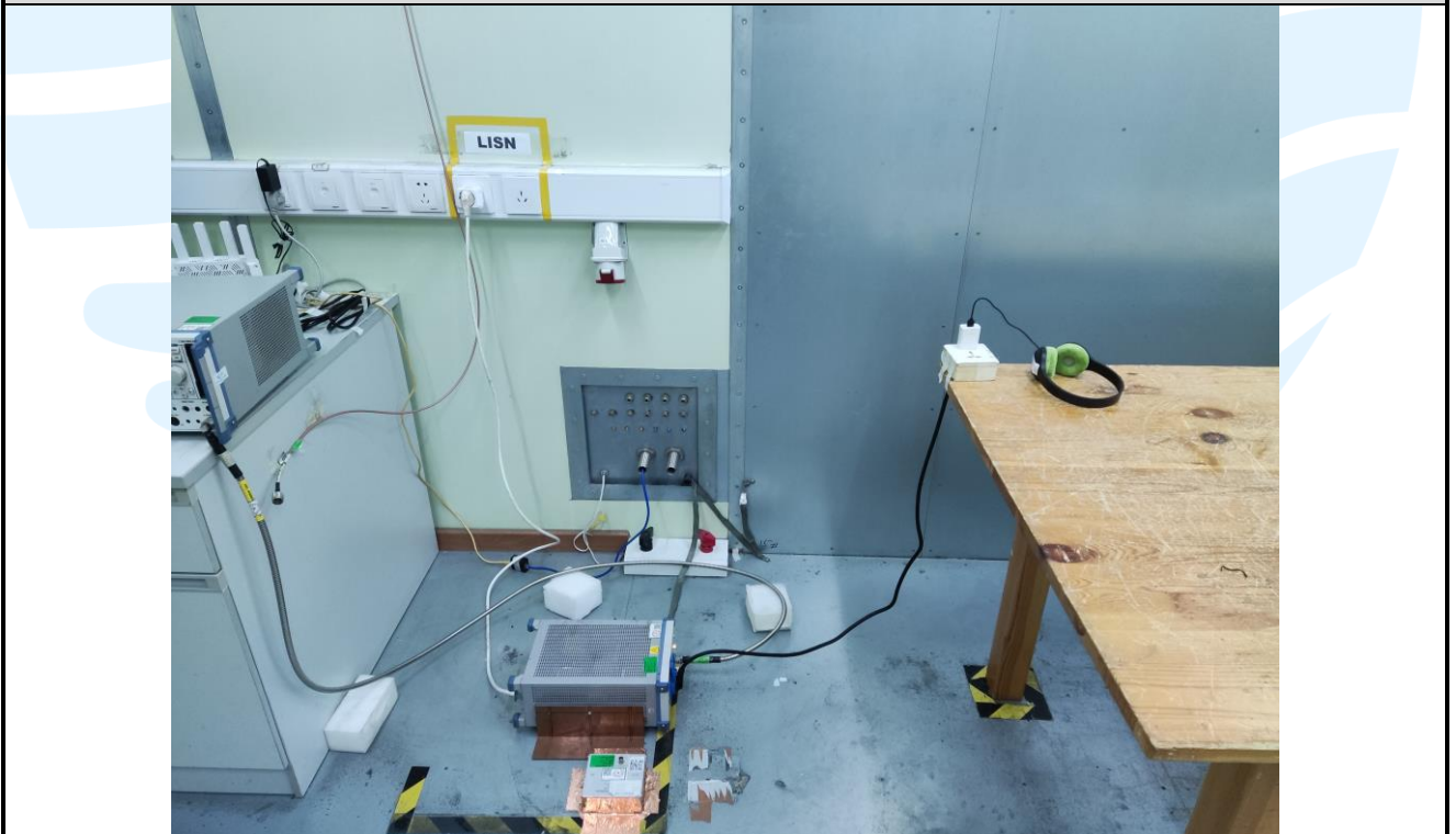
Conducted Emission Test Setup
