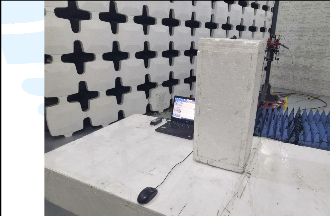
Radiated emission Test Setup (Above 1 GHz)
