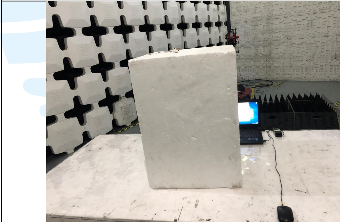
Radiated emission Test Setup (Above 1 GHz)
