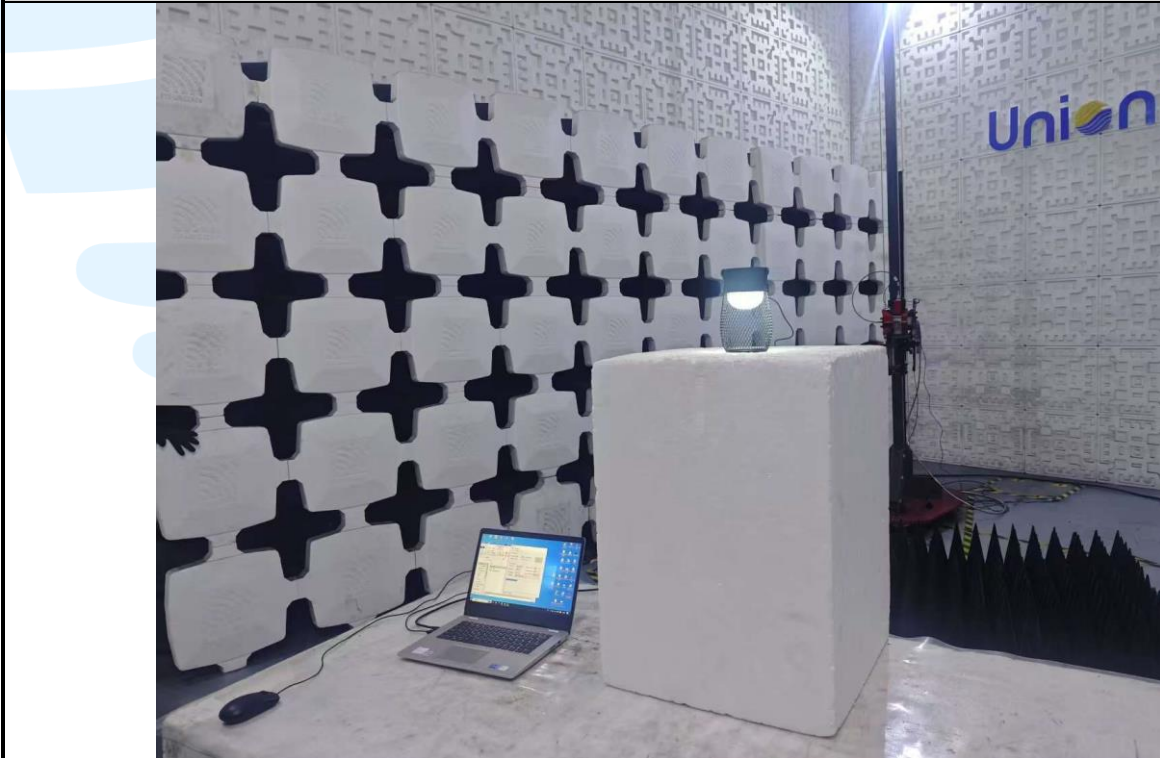
Radiated emission Test Setup (Above 1 GHz)
