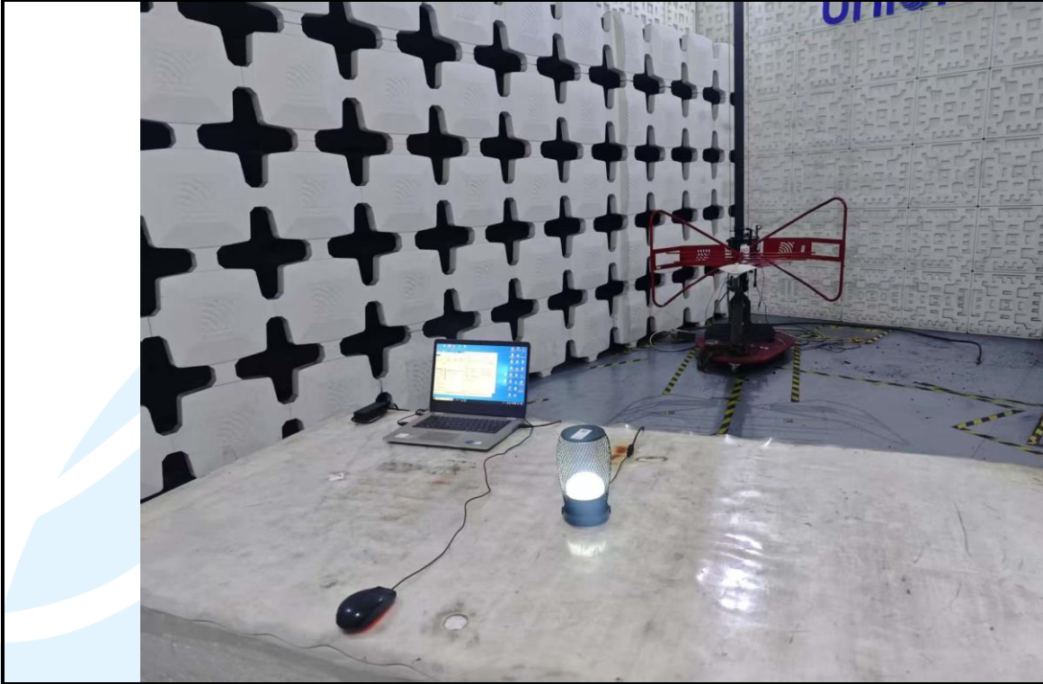
Radiated emission Test Setup (30 MHz~1 GHz)
