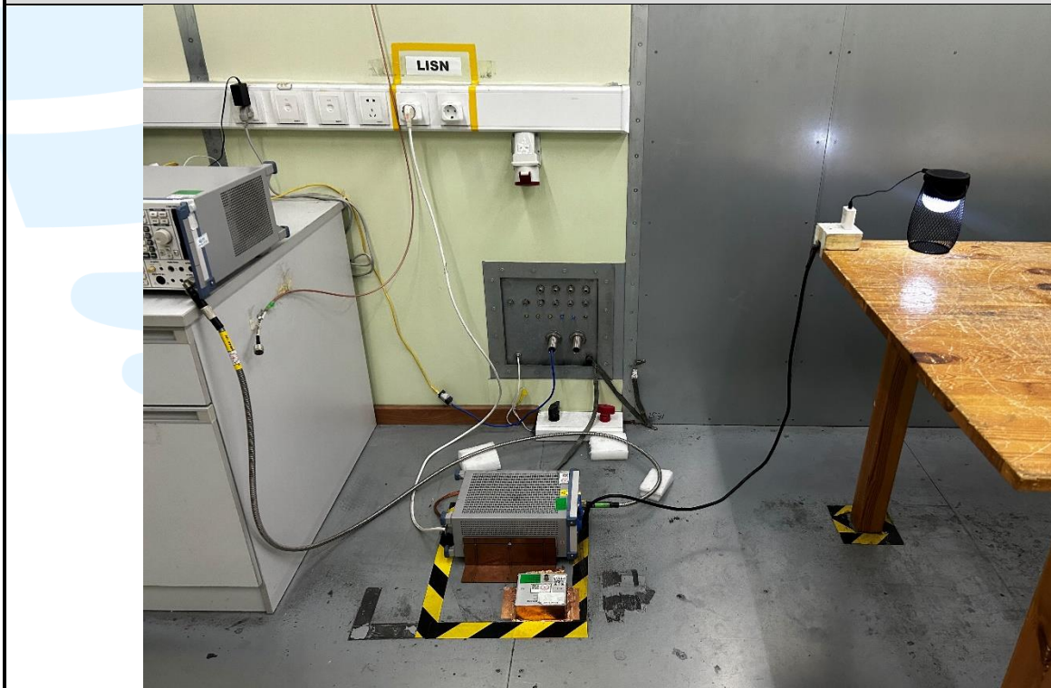
Conducted Emission Test Setup
