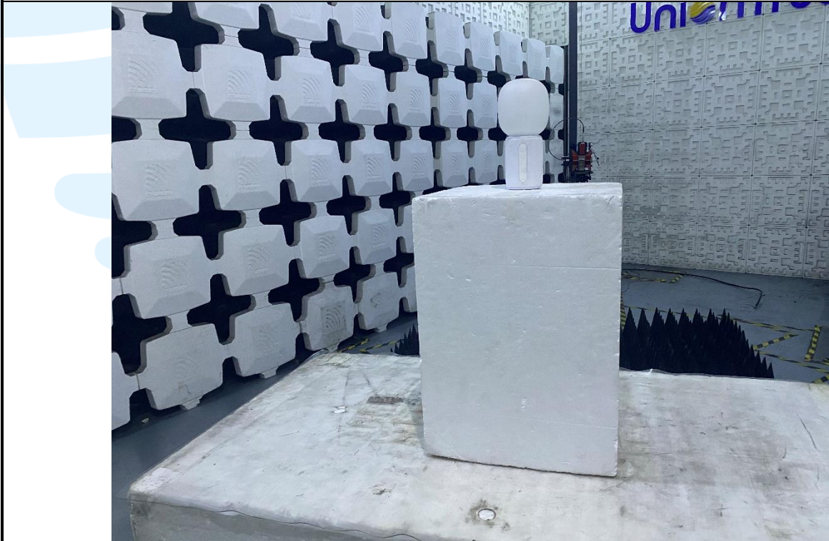
Radiated emission Test Setup (Above 1 GHz)
