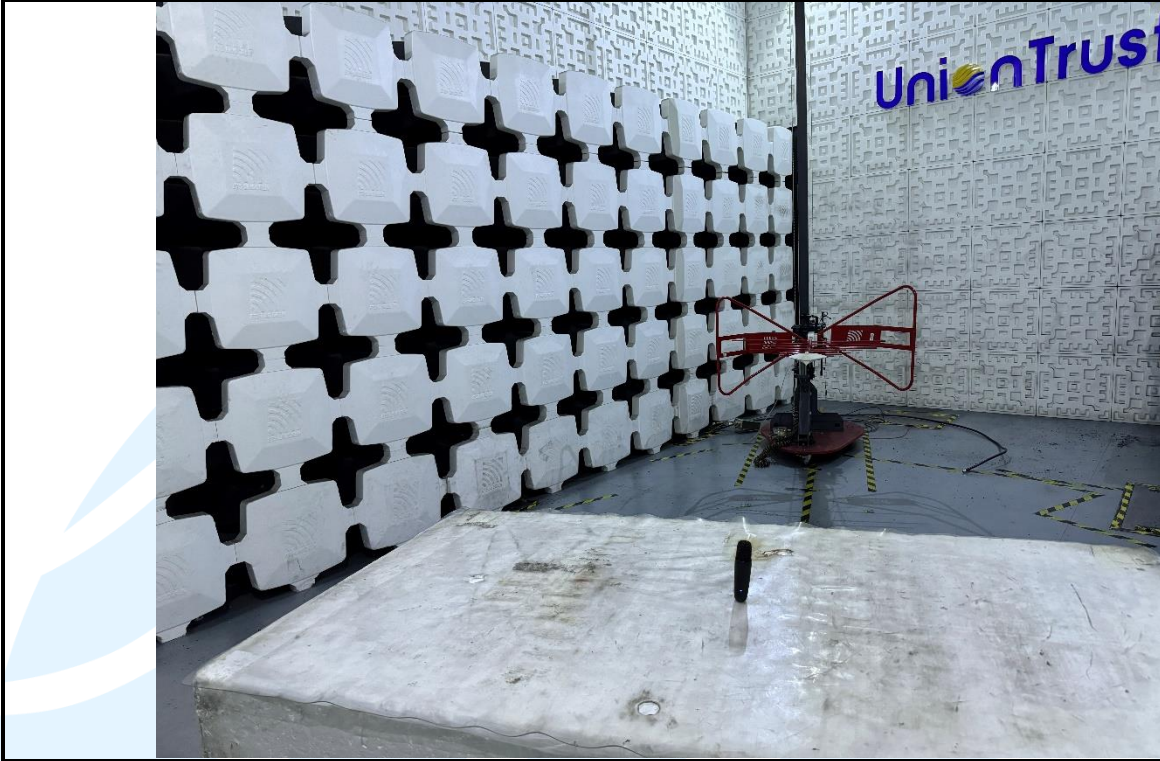
Radiated emission Test Setup (30 MHz~1 GHz)
