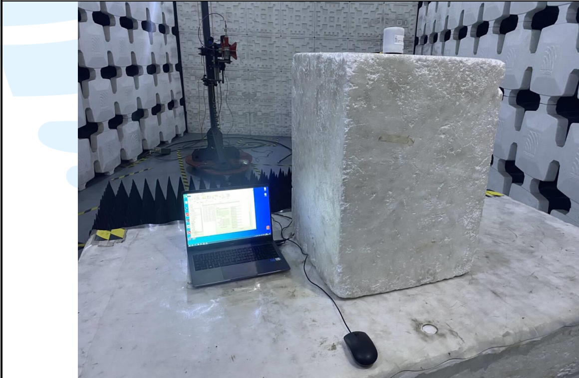
Radiated emission Test Setup (Above 1 GHz)
