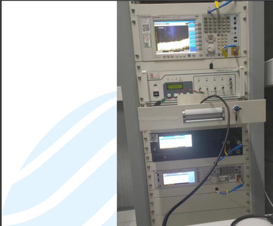
RF Conducted Test Setup
