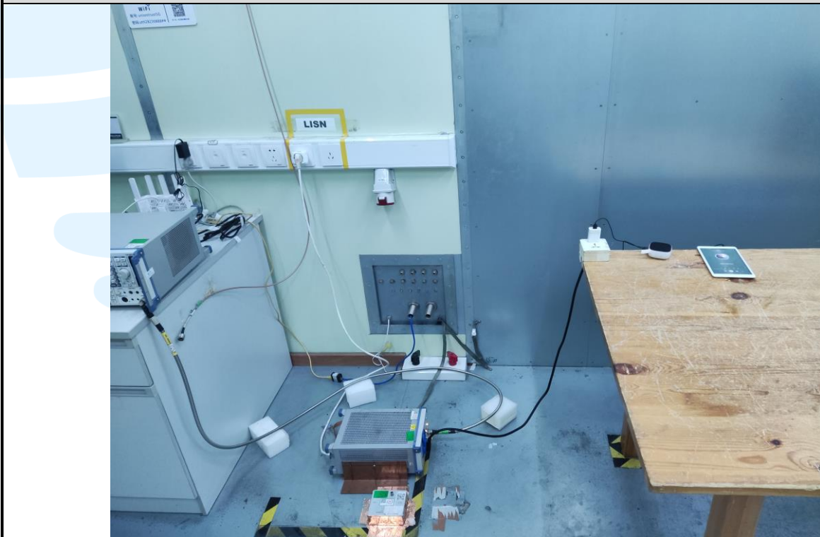
Conducted Emission Test Setup
