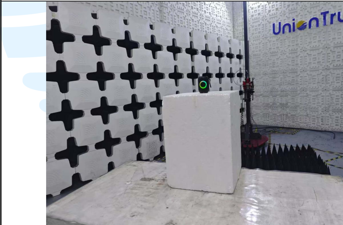
Radiated emission Test Setup (Above 1 GHz)
