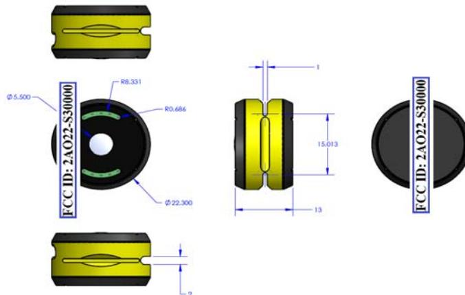
It is difficult to apply ISEDC and FCC ID on a device due to small size and mechanical structure of the device.
