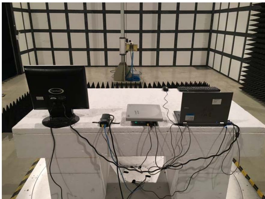
Radiated Disturbances Rear Side (Above 1GHz )
