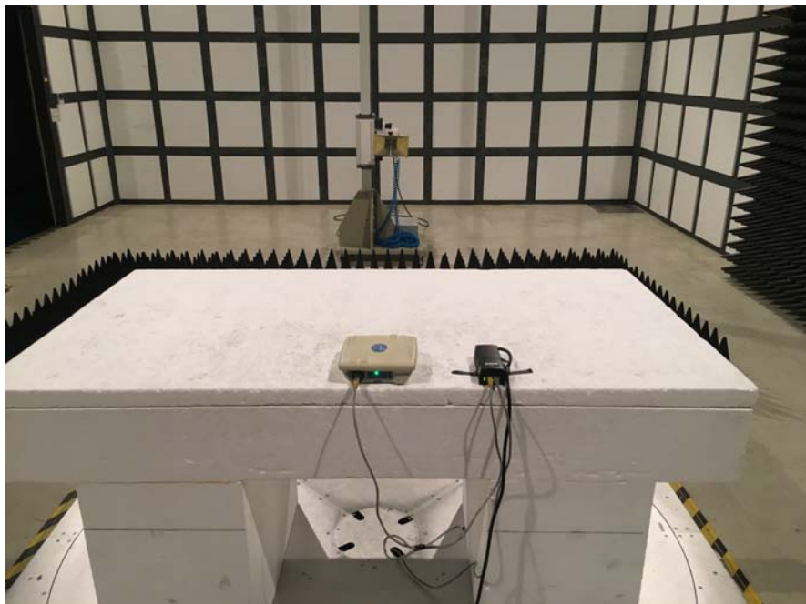
Radiated Disturbances Rear Side (Above 1GHz )
