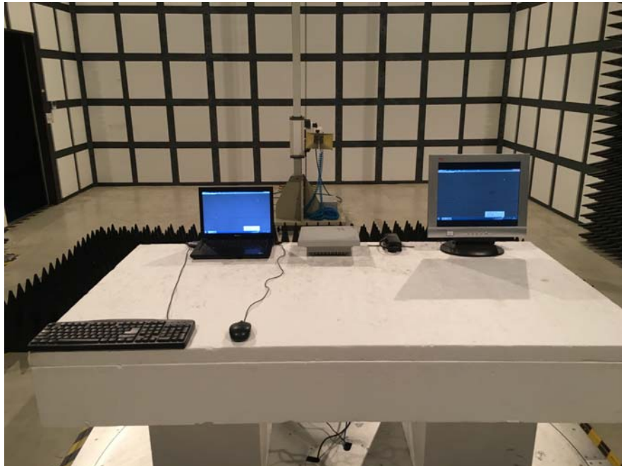
Radiated Disturbances Rear Side (Above 1GHz )
