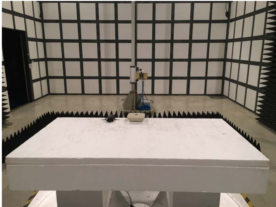
Radiated Disturbances Rear Side (Above 1GHz )
