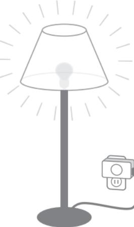
Plug lamps into configured Switcheroos™ as desired. The "Send" unit does not need to have a lamp plugged into it for the system to work.
