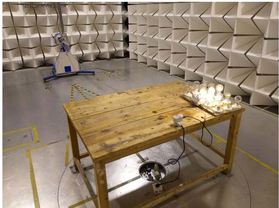
Test frequency 1GHz to 10GHz
