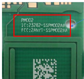
Figure 4 Apperance of test writing of FCC/IC label written on PCB for PM002
