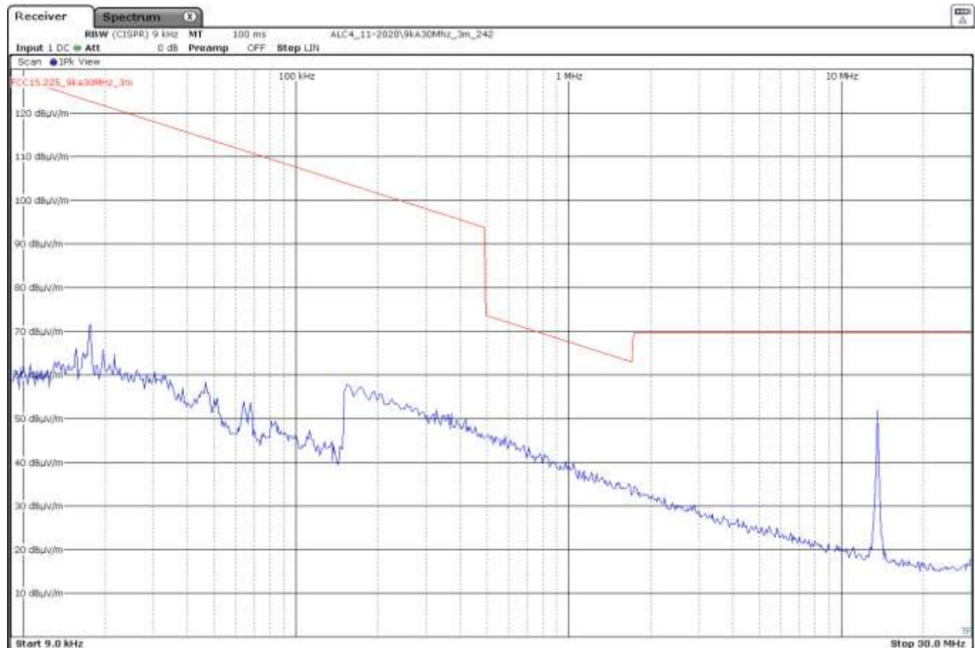
The limits shown in this plot are extrapolated to 3 m. The highest peak is the carrier frequency.
