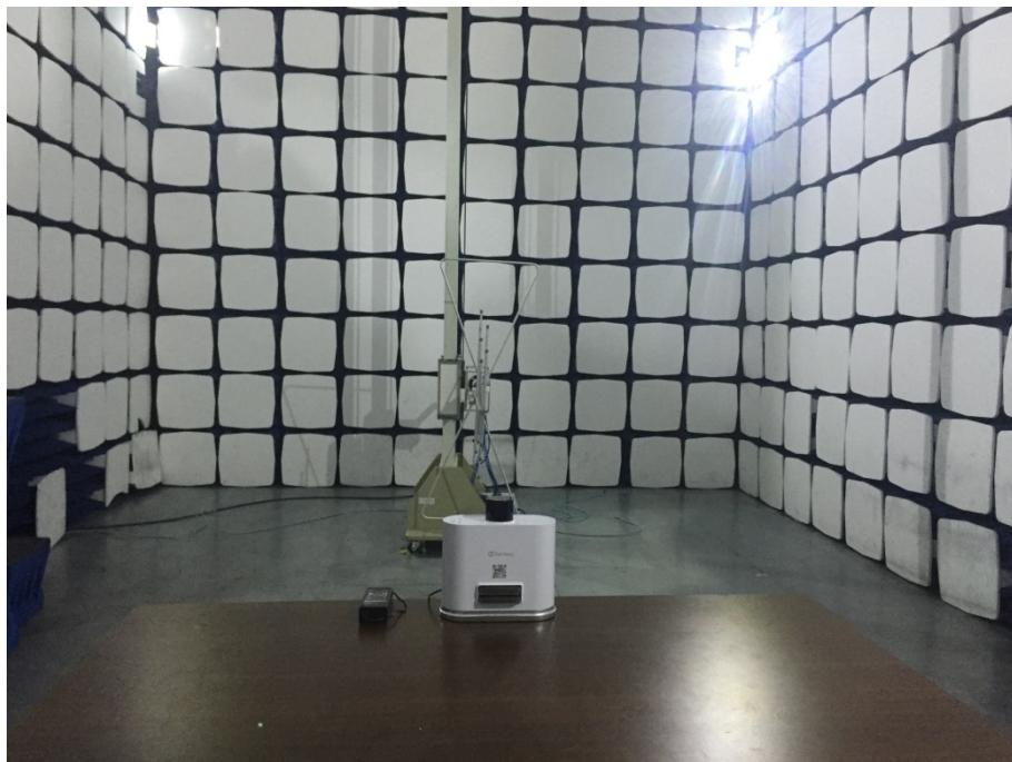
**Radiation Emission Test Setup (above 1GHz)**
