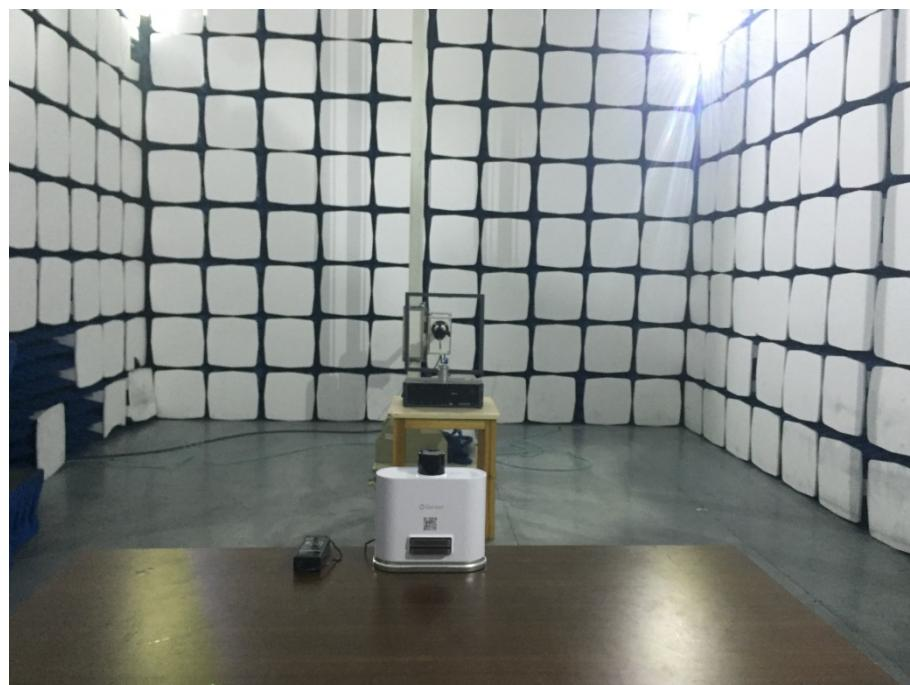
**Radiation Emission Test Setup (30MHz to 1GHz)**
