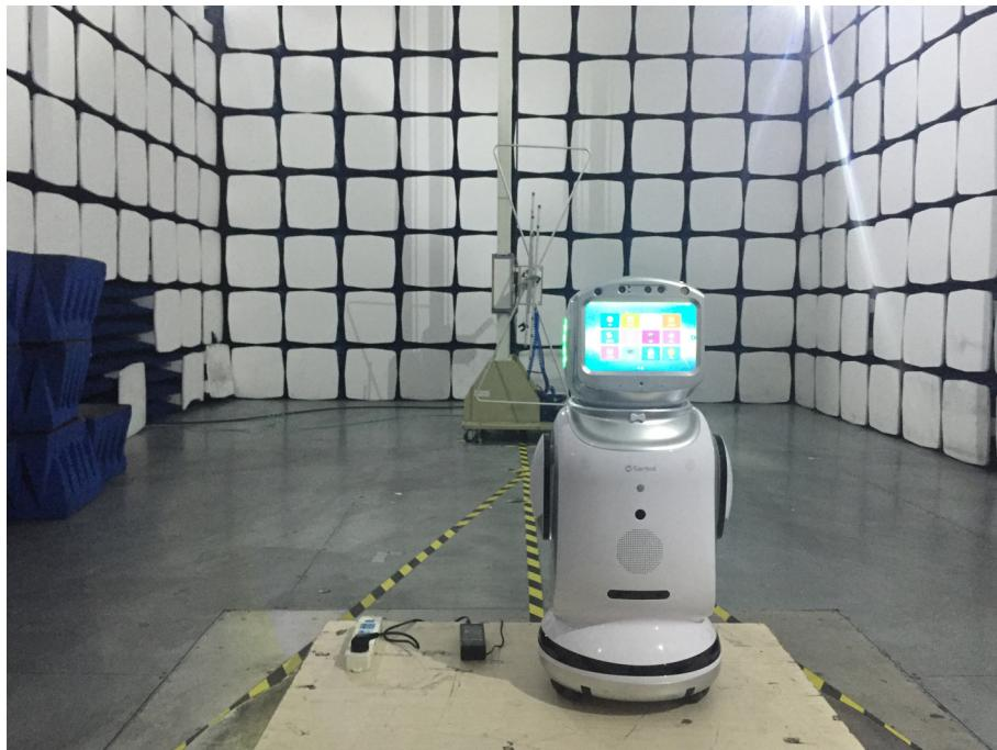
**Radiation Emission Test Setup (Above 1GHz)**
