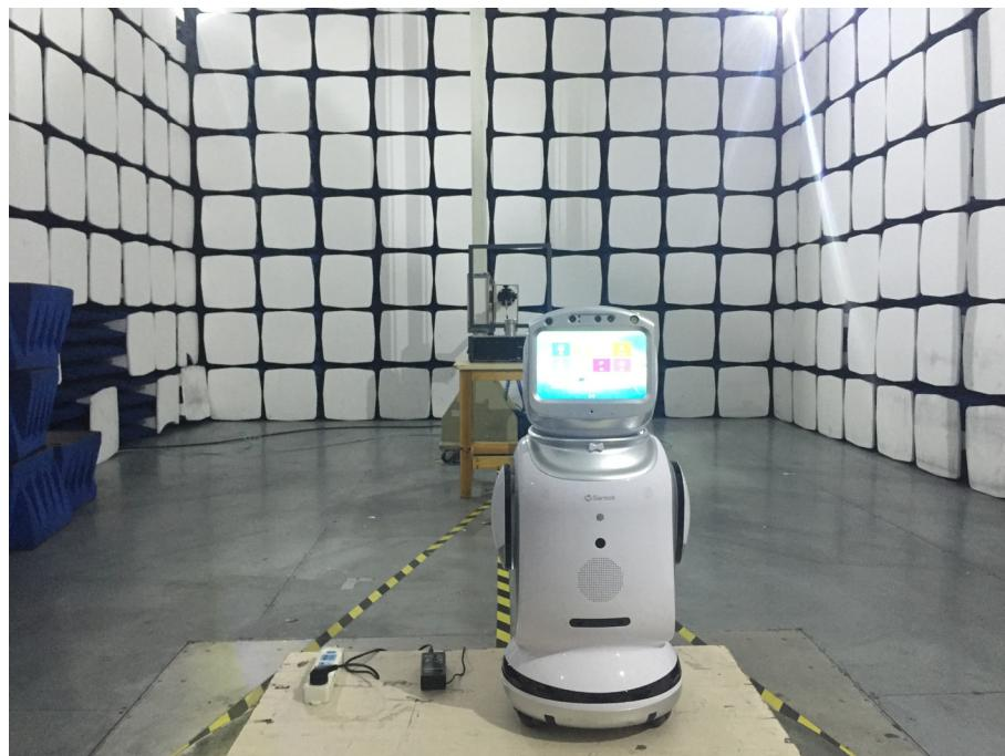
**Radiation Emission Test Setup (30MHz to 1GHz)**
