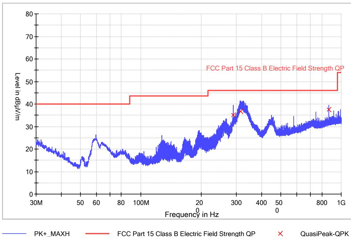
— PK+\_MAXH — FCC Part 15 Class B Electric Field Strength QP X QuasiPeak-QPK (Single)
