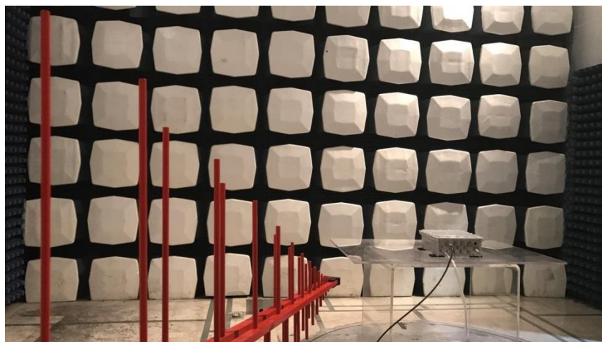
Photograph 1. Radiated Spurious Emissions, Test Setup (Below 1GHz) (A)
