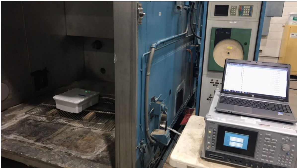
Photograph 6. Frequency Stability, Test Setup (B)
