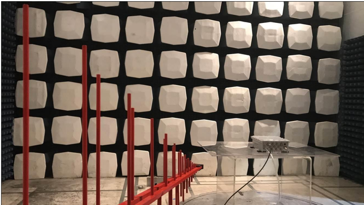
Photograph 4. Radiated Spurious Emissions, Test Setup (1) (B)
