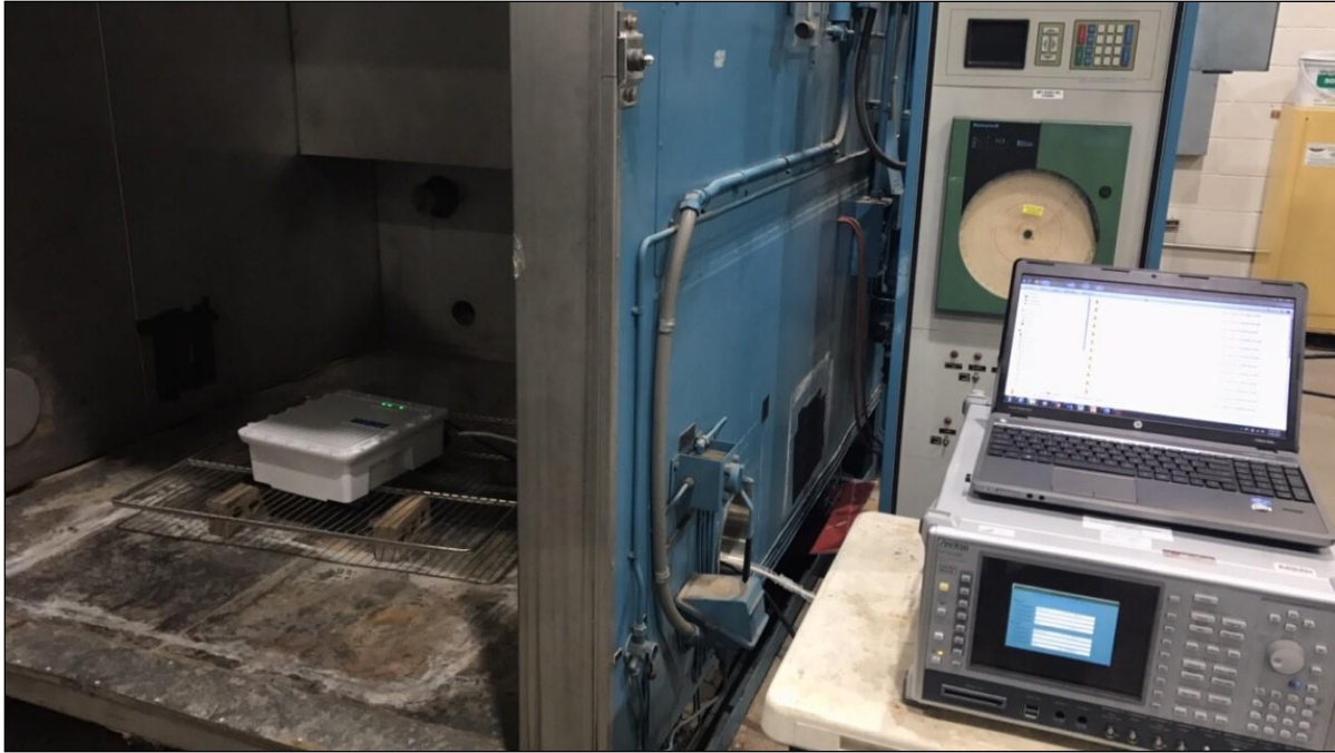
Photograph 3. Frequency Stability, Test Setup (A)
