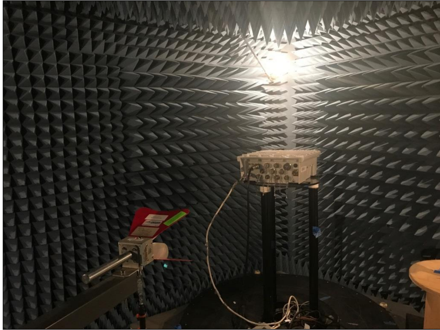
Photograph 5. Radiated Spurious Emissions, Test Setup (2) (B)
