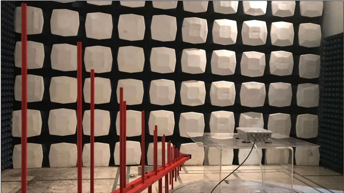
Photograph 1. Radiated Spurious Emissions, Test Setup (1)
