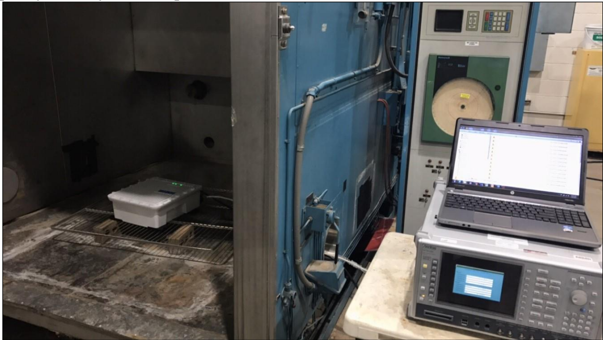
Photograph 3. Frequency Stability, Test Setup
