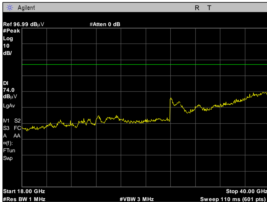
Plot 80. Simultaneous Transmission LTE WiFi 18-40 GHz Peak
