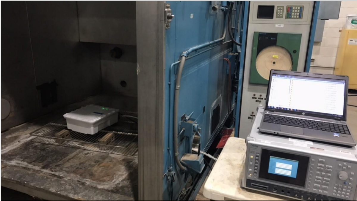
Photograph 3. Frequency Stability, Test Setup
