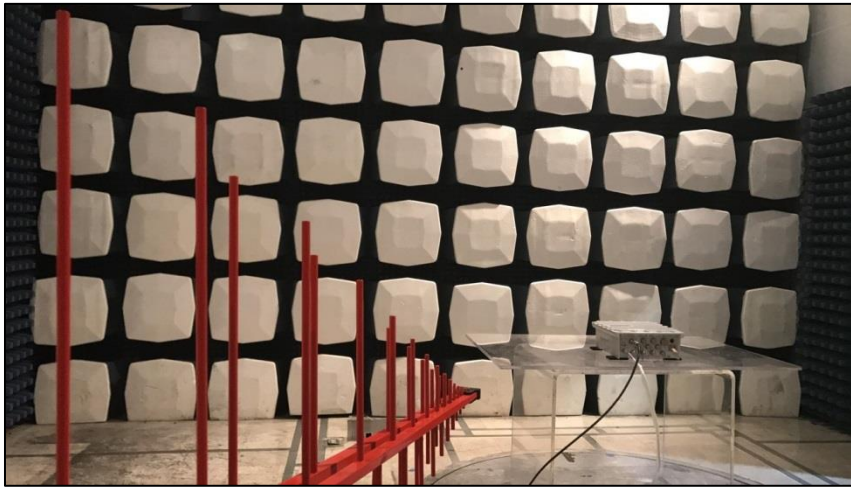
Photograph 1. Radiated Spurious Emissions, Test Setup (Below 1GHz)
