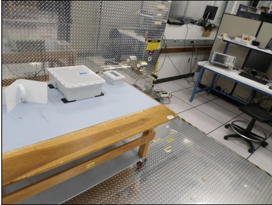
Photograph 10. Conducted Emissions, 15.207(a), CEV Station Setup
