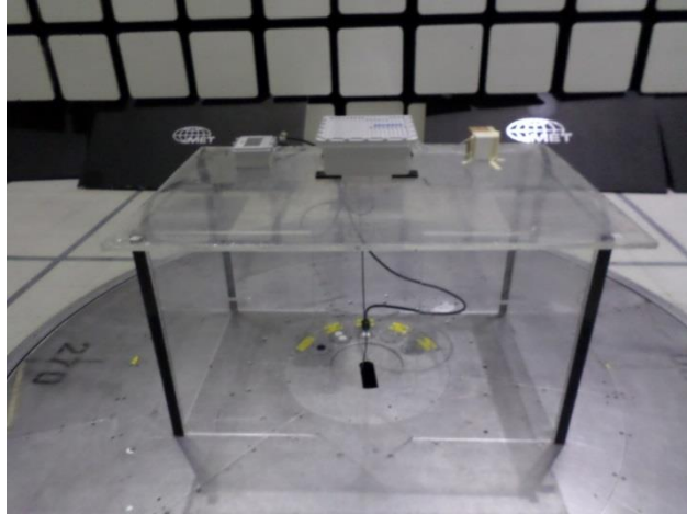
Photograph 1. Radiated setup, 30M-1GHz front view
