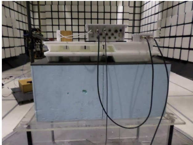
Photograph 5. Radiated setup, 1-18GHz rear view
