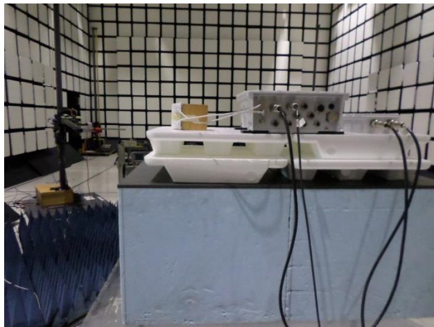
Photograph 8. Radiated setup, 18-40GHz rear view
