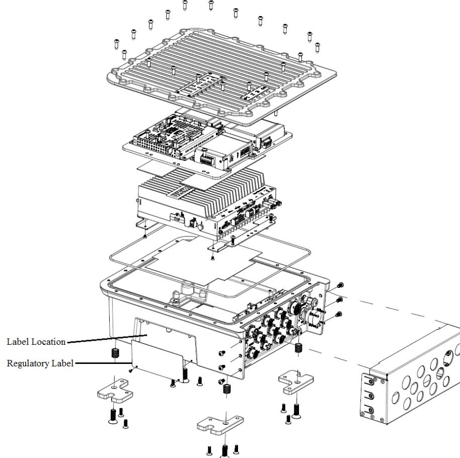
The MPM's regulatory label shall be mounted on the side of the enclosure in the recess shown in the figure. The label is secured using two M3x5 screws.
